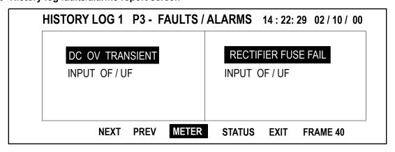
As previously mentioned, faults are shown in reverse video, and alarms in regular video. For a complete list of all the alarm messages and corrective actions for these faults, refer to **Table 7 - Alarms**, **functions**, **and corrective actions**.
